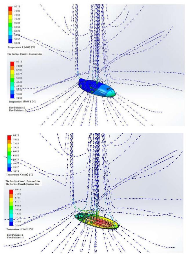
• Use FLOEFD software to simulate the lamp heat dissipation condition, analyze the construction of lamp heat dissipation, thus to achieve the best effect of heating dissipation.
