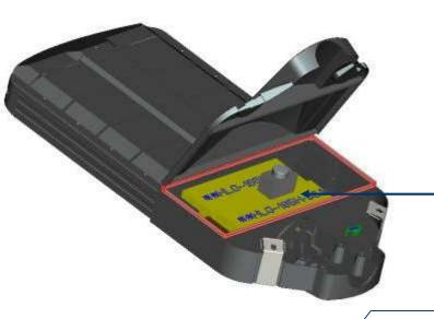
Drivers are mounted in their most thermally efficient position, upside down on the door which is acting as a heat sink. This mounting position greatly improves electronics cooling.
